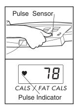
**tected.** Next, raise your thumb slightly until the heart-shaped indicator in the pulse display flashes **steadily**. Hold your thumb at this level. After a few seconds, three dashes will appear in the display and your pulse will be shown. Hold your thumb on the sensor for another 15 seconds for the most accurate reading.
